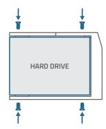
4. Insert and screw the bracket back to S380 HomeBase, then put the top lid back into place.
