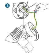
To avoid risk of shock,injury or death, always be cautious when working with electricity. Remember, do hire a professional electrician if you're uncomfortable working with electrical wiring. 3. Use wire nuts to connect Floodlight Cam wires to the rest of the wires from junction box. Connect the white wire on the Floodlight Cam to the white wire(neutral) from junction box. Connect the black wire on the Floodlight Cam to the black wire(hot) from junction box.
